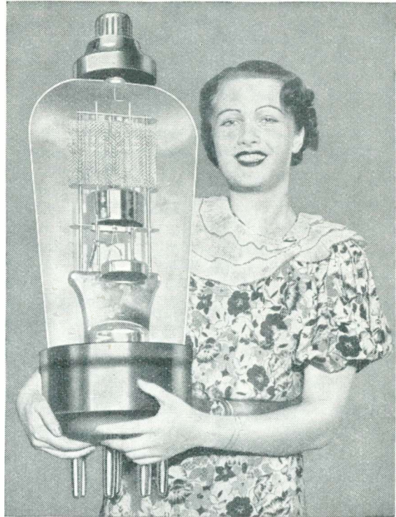
The author suggests that you use a screen-grid valve as a diode detector—something on the lines of this G.E.C. model.
