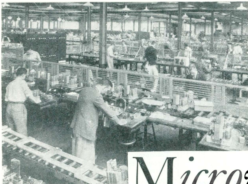
Part of the extensive radio test section of the vast Coventry works of the G.E.C., which turns out two radio sets every minute
